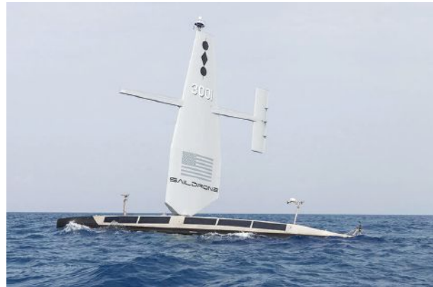
THE SAILDRONE SURVEYOR USV is a purpose-built platform for autonomous deep-water ocean mapping.
